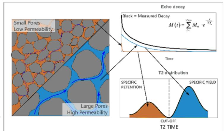
**The total BMR measured echo delay is the sum of the contribution from a range of different pores in the measured region. The inversion process to T2 time solves for the amount of porosity associated with a particular T2-time, resulting in the pore size (T2) distribution**
